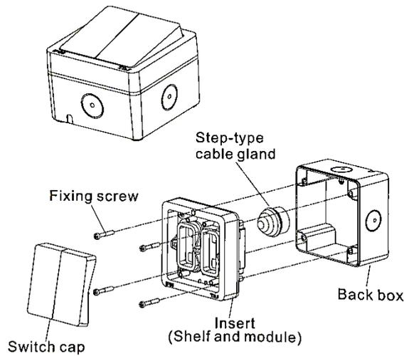
**Note:** When re-installing switch cap, observe orientation, left or right cap and in “up” position.
