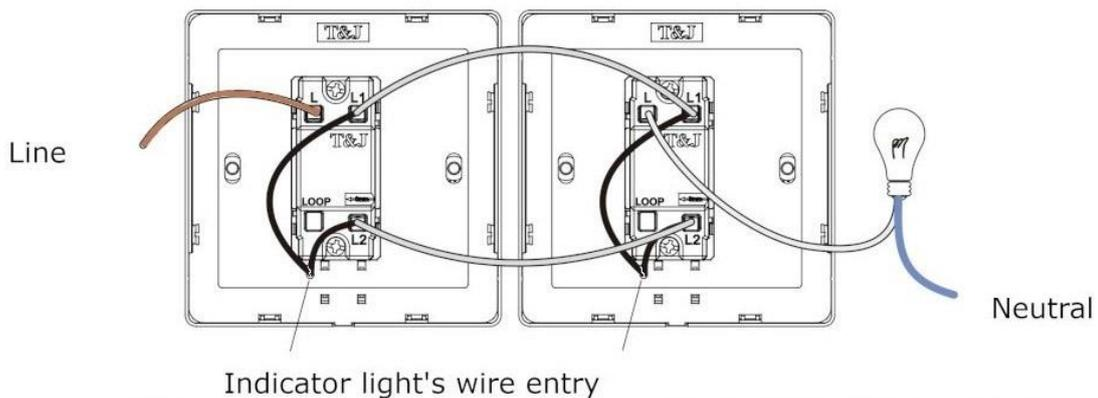
\*This connection may not work for low wattage (<5W) LED lamp load, the lamp may appear dimly lighted even if switched off.
